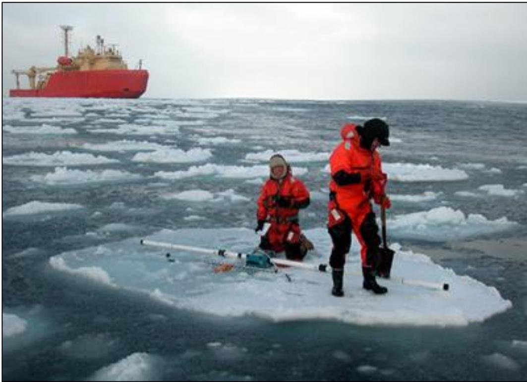
Figure 3. Researchers measuring the sea ice thickness of small ice floes during the West Antarctic Sea Ice Campaign. The research ship Lawrence M. Gold is shown in the background. Image courtesy of Dr. Konrad Steffen. All rights reserved.
