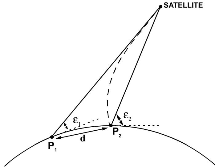
Figure 3. Geometry of laser ray path.
