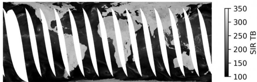
Figure 3. Temperate grid sample image from file NSIDC-0630-EASE2_T6.25km-AQUA_AMSRE-2011270-18H-A-SIR-RSS-v1.3.nc. The image shows 18 GHz H-polarized TB (in Kelvin) at 6.25 km Enhanced Resolution; TB was derived using the rSIR method.
