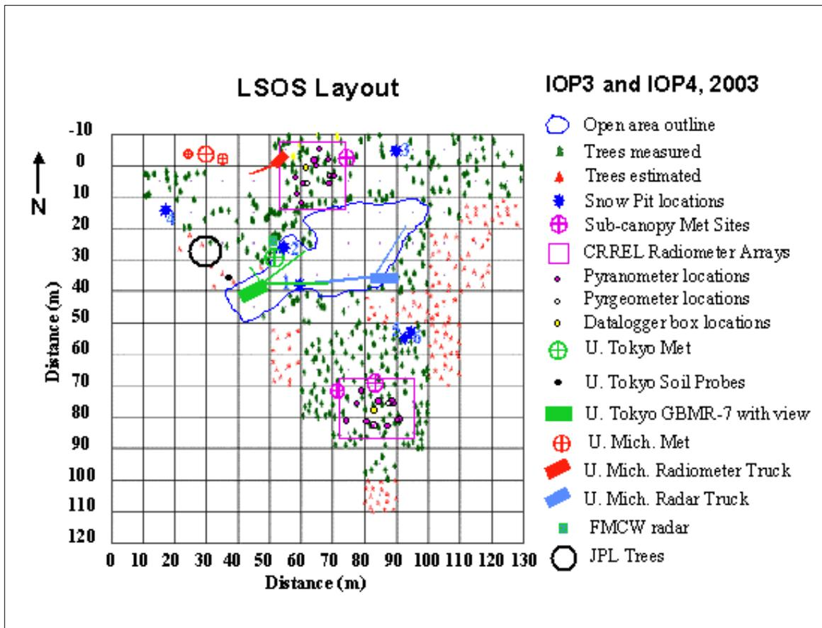
Figure 3. LSOS Layout in IOP3 and IOP4 (2003)
