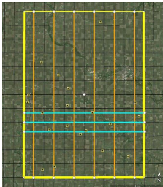
Figure 2. PALS flight lines drawn on Google Earth. High-altitude (3000 m) mapping lines are marked with orange and the low-altitude (1200 m) high resolution lines are marked with light blue. Also shown is the validation grid (yellow) and permanent in situ soil moisture stations.
