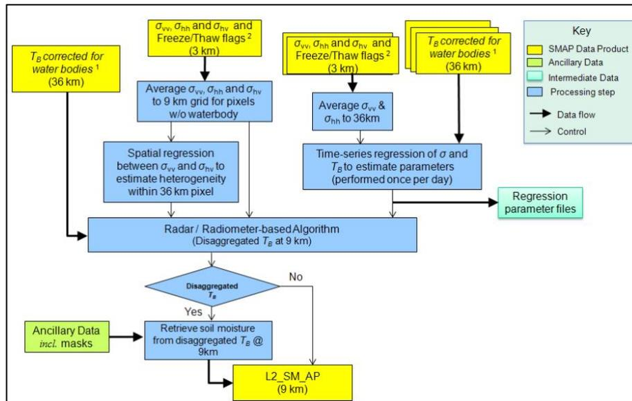
Figure 4. Process Flow Diagram of the Baseline SPL2SMAP Algorithm
