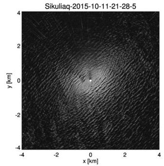
Rutter radar raw image of wave signal within the pancake ice
