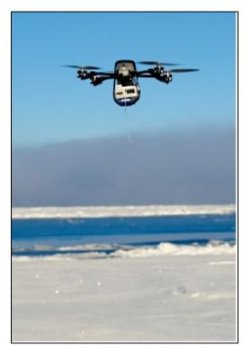
InstantEye UAS with radiosonde attached below
