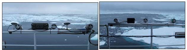
Port Side Stereo Cameras and IMU
