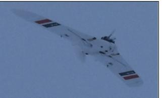
Fixed wind UAS with radiosonde on top.
