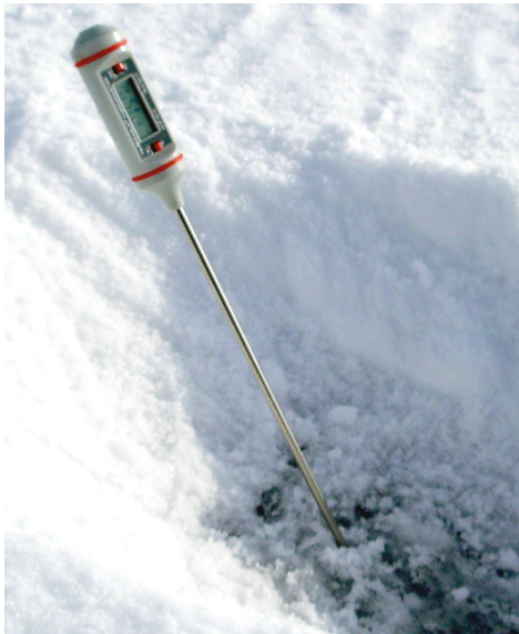
Above left: A digital thermometer inserted into a hole at a 45-degree angle to measure surface sea ice temperature (Section 4.3 and Figure 12). Above right: A digital thermometer inserted horizontally into the snow 5 cm from the ice surface (Section 4.4 and Figure 12). Photos: Nina Palituq
