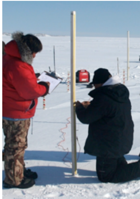
Above left: A hotwire gauge with handle hanging on nail above the snow. Photo: Teema Qillaq. Above right: Toku Oshima and Teema Qillaq pull up on a heated hotwire cable and measure the length of the cable, as described in Section 3.3. Photo: Andy Mahoney
