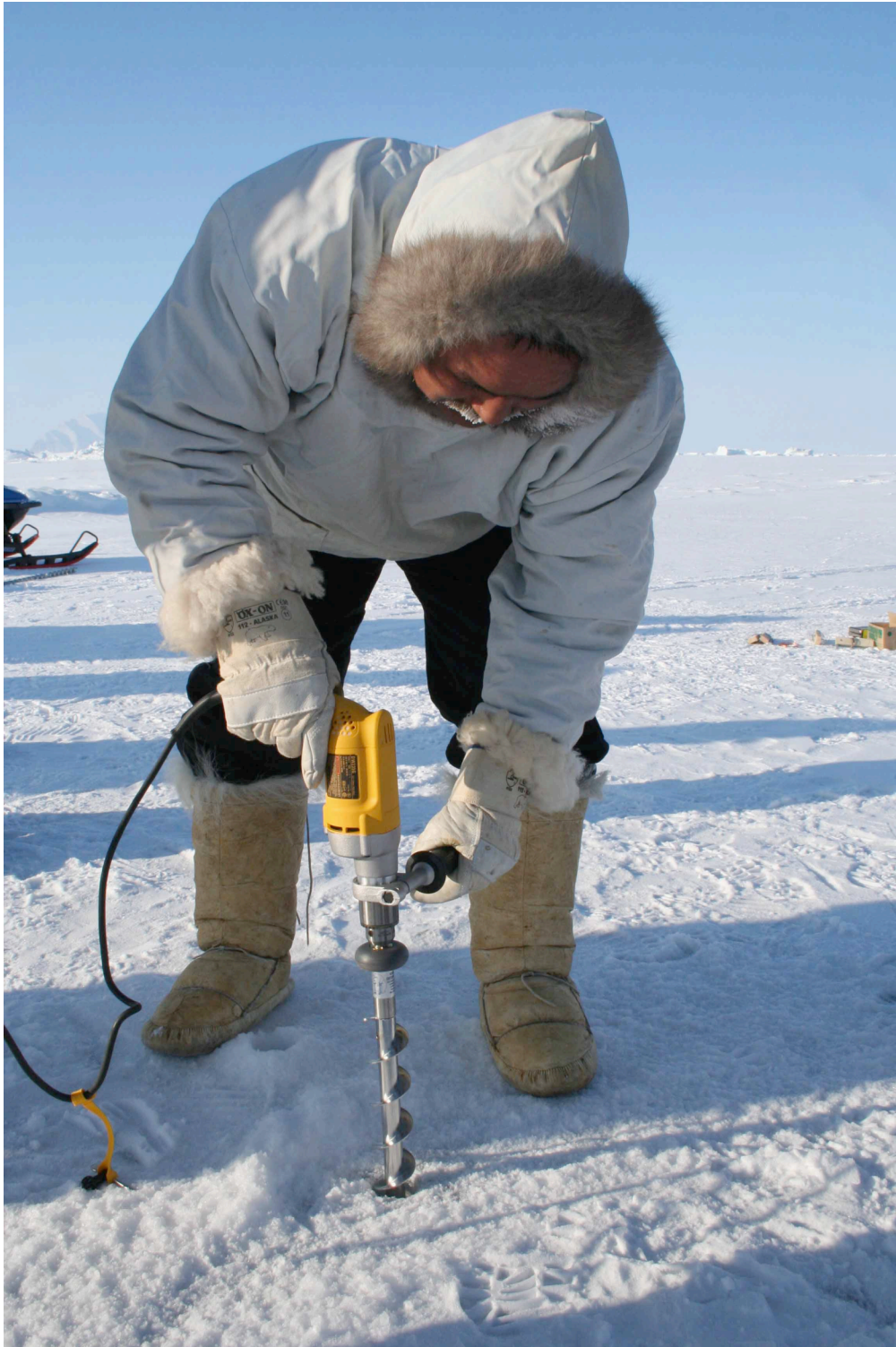
Mamarut Kristiansen of Qaanaaq, Greenland demonstrates the Kovacs auger attached to an electric drill, powered by a generator. The drill is a quick and easy way to measure sea ice thickness with measuring tape (Chapter 1) and install the permanent stakes of the monitoring stations (Chapter 2). Photo: Shari Gearheard
