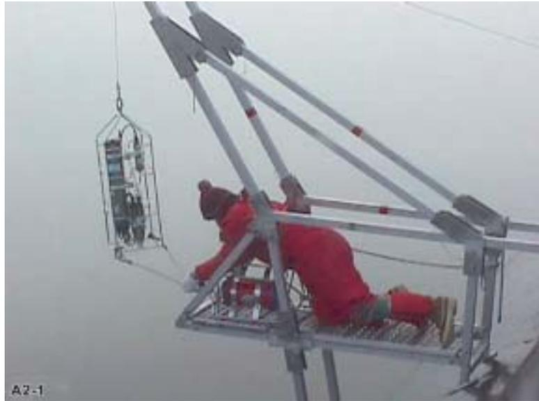
**Fig. A2-1.** Jay Ardai (LDEO) launches an Acoustic Doppler Current Profiler from the deck of the *USS Hawkbill* during SCICEX-98. The winch and gantry used for surface casts during this cruise were provided by ASL. Photo: Greg Kurras.
