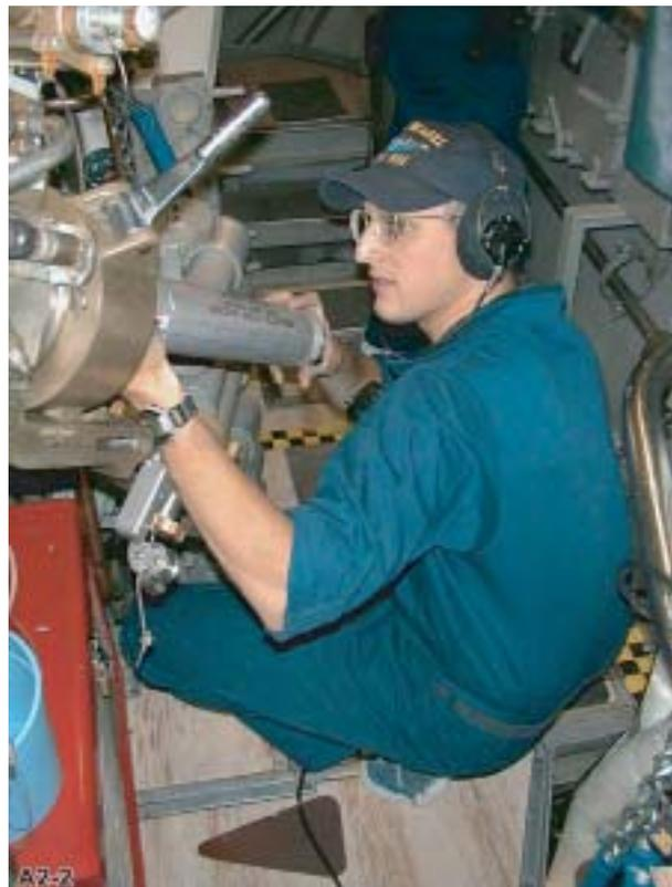
**Fig. A2-2.** Crewman “Ted” Groustra loads an SSXCTD for launching. These instruments were designed to measure physical and chemical water properties under the arctic ice canopy. Their operation is described in the text. Photo: ASL.
