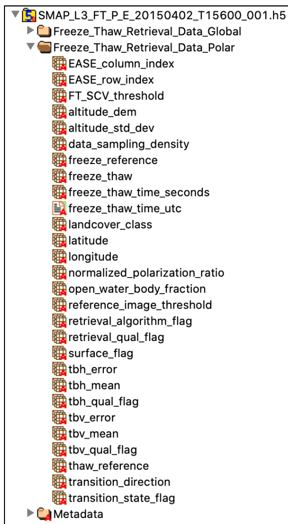
Figure 1. Subset of File Contents. For a complete list of file contents for the SMAP enhanced Level-3 radiometer freeze/thaw product, refer to the Appendix – Data Fields Section in this document.
