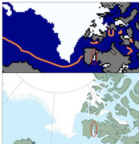
Figure 21. Screenshots of the Sea Ice Index daily extent (top) and MASIE daily extent (bottom) from 08 September 2011. The red ellipses show one area, between Banks Island and Victoria Island, where SII and MASIE differ significantly. MASIE is the more accurate product because of the visible band data used as input.
