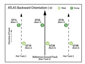
Figure 1. Spot and ground track (GT) naming convention with ATLAS oriented in the forward (instrument coordinate +x) direction and backward (instrument coordinate -x) direction.
