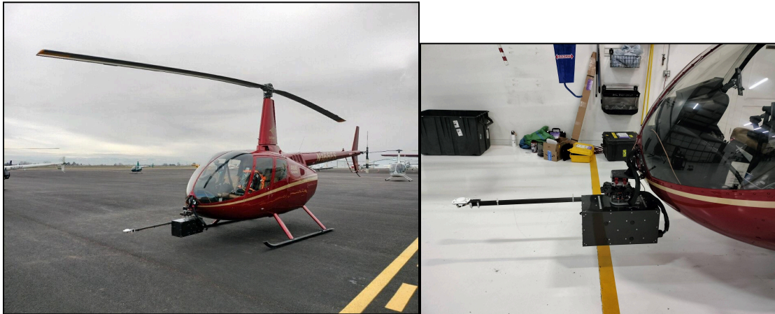
Figure 2 - CRREL's nose-mounted RaLiPod system installed on a Robinson R66 helicopter. All sensors are located inside the pod, with control systems located within the passenger compartment for in-flight operations.
