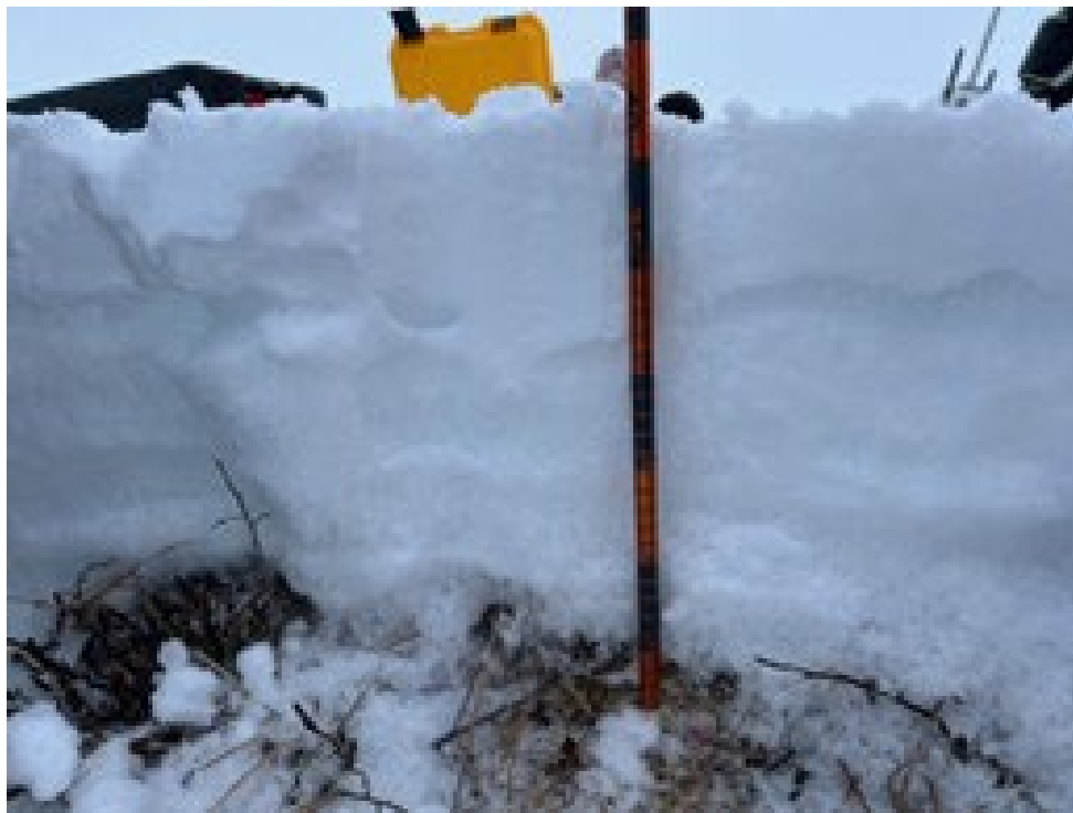
Figure 2. Excavated snow depth profile showing depth probe sinking into soft organic layer underneath the snowpack (example from Arctic tundra, UKT study area). The distance between snow-vegetation interface and impermeable (for snow depth probe) mineral soil is 12 cm. The depth profile data was adjusted to remove this overprobe error.
