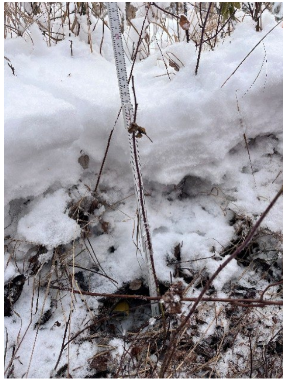
Figure 1. Example air gap beneath the blanket of snow caused by grass supporting the snow above. Photo taken by Megan Mason.
