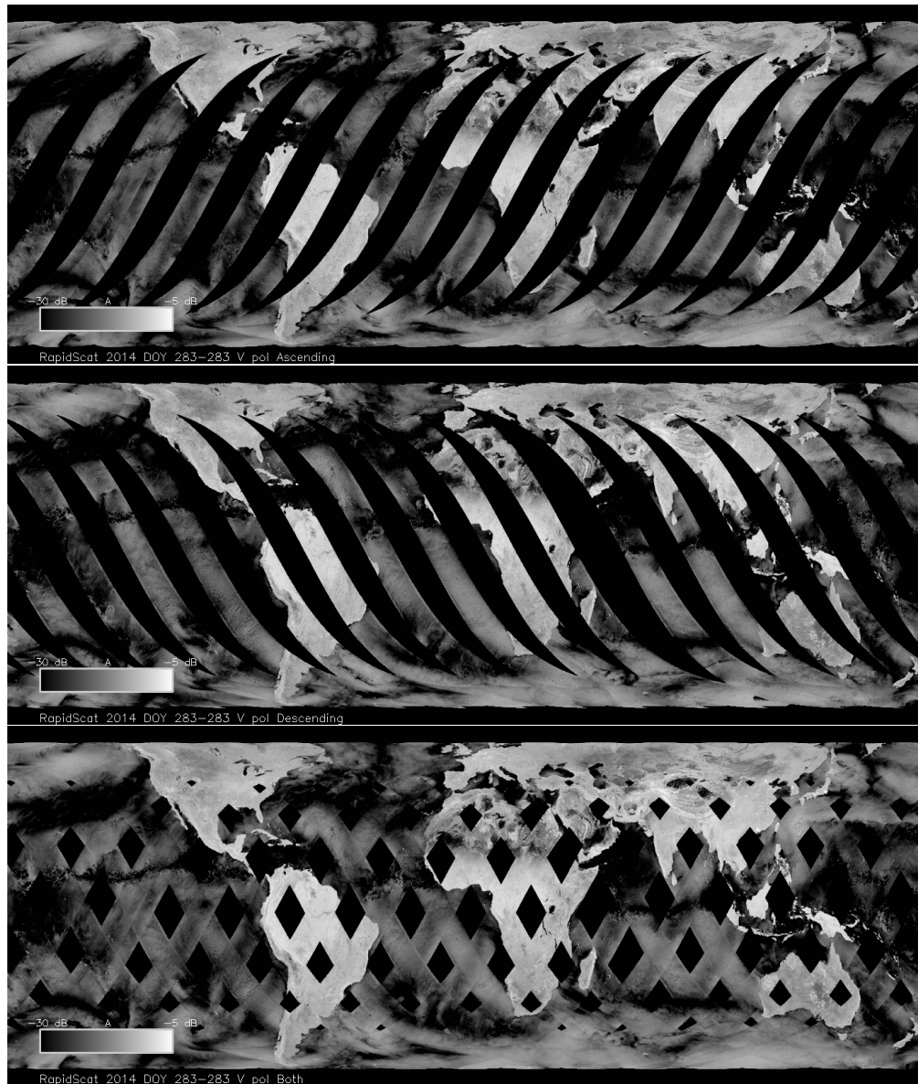
Figure 11: Example 1-day RapidScat VV-polarization \sigma^0 images for DOY 283: (top) ascending, (center) descending, (bottom) both passes. Image resolution has been reduced for display.
