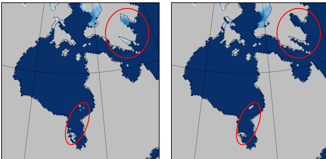
Figure 5. Differences in the effectiveness of NT (left) and NT2 (right) land-spillover corrections for 13 August 2023. The areas circled in red show areas of ice not removed by the NT algorithm (left) but that are removed by the NT2 algorithm (right).
