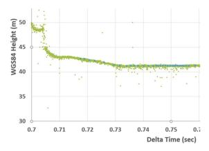
Also, some coastal buffer of narrow inlets and bays caused swaths of land to be included in version 3 of the ATL13 Inland Water Body Mask. In these cases, it is possible that flat land will create enough of a histogram signal to compel the algorithm to process the crossing as if it were water (See example below).
