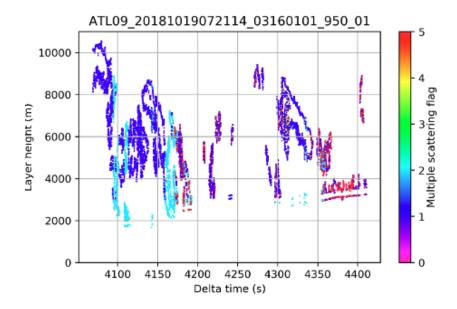
As shown in the ATLO3 example above, the photon cloud can at times be denser below the surface than above. The phenomenon is due to multiple scattering and can occur over surfaces with heavy blowing snow, such as the example shown here, or over dense fog. Such conditions result in a widening of the surface return, and more photons apparent below the surface. The effect of multiple scattering is more prominent at night when the solar background signal is absent.
