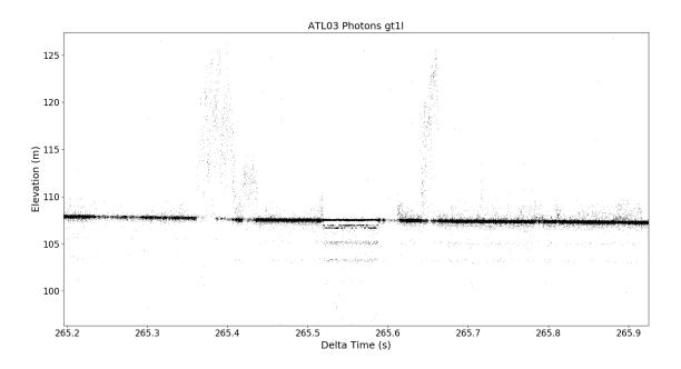
Over flat water, at times the returning laser light will be specular or nearly so. In these cases, the returning laser light will have had minimal pulse spreading and minimal energy loss from light scattering out of the receiver field of view. The returning pulse is therefore narrower and stronger than ATLAS was designed to handle. In these circumstances (e.g. 265.5 to 265.6 seconds), ATLAS detects multiple surface returns, with echoes spaced by either one or two times the ATLAS dead time.
