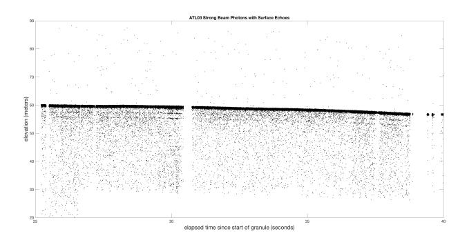
Over relatively flat surfaces, when plotting ATL03 as along track distance or time, double echoes are sometimes seen at ~2.3m below the primary surface and ~4.2m below the primary surface return. The amount of energy in these additional horizons are typically 1/1000 of the energy in the surface echo. The double echoes appear visually prominent in plots, such as above, because all of the surface return photons are stacked on top of one another, given little changes in photon density.
