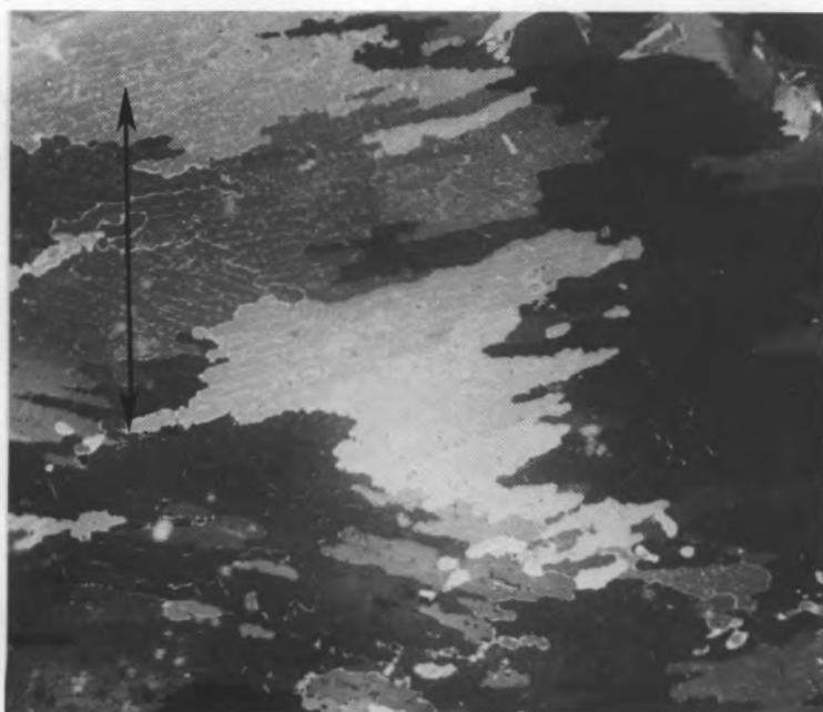
Figure B1 (cont'd). Horizontal thin sections demonstrating retexturing in the upper levels of a multi-year ice floe (site 6-15-1). Note in section from 90 cm that original c-axis alignment (arrow) is maintained despite nearly complete loss of brine pocket substructure. Smallest scale subdivision measures 1 mm. Same scale applies to all four sections.
