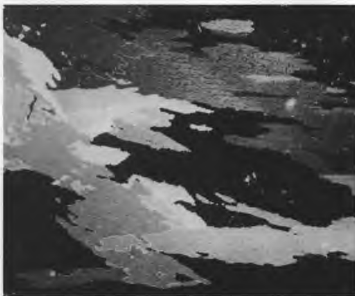
a. Strongly aligned c-axes (normal to platelet structure) from 203-cm depth.
