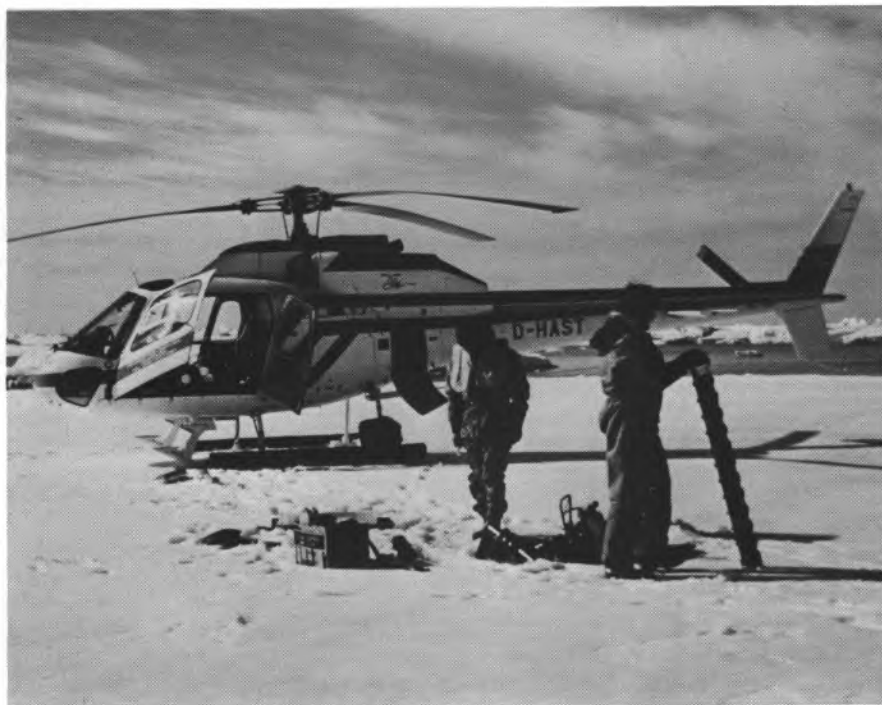
Figure 2. Setting up coring site on multi-year floe with aid of helicopter.
