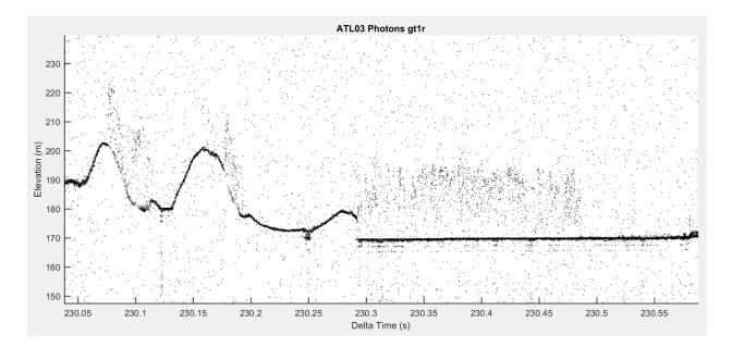
Over flat water, at times the returning laser light will be specular or nearly so. In these cases, the returning laser light will have had minimal pulse spreading and minimal energy loss from light scattering out of the receiver field of view. The returning pulse is therefore narrower and stronger than ATLAS was designed to handle. In these circumstances (e.g. 230.3 to 230.55 seconds), ATLAS detects multiple surface returns, with echoes spaced by either one or two times the ATLAS dead time.
