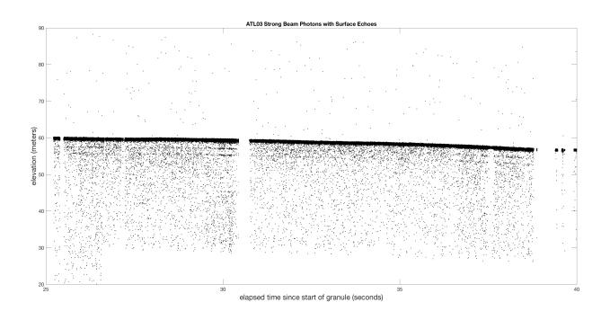
Over relatively flat surfaces, when plotting ATL03 as along track distance or time, double echoes are sometimes seen at ~2.3m below the primary surface and ~4.2m below the primary surface return. The amount of energy in these additional horizons are typically 1/1000 of the energy in the surface echo. The double echoes appear visually prominent in plots, such as above, because all of the surface return photons are stacked on top of one another, given little changes in photon density.
