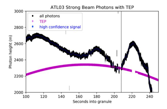
The example above has all telemetered photons in the ATL03 granule (black), high-confidence signal photons (blue) and an obvious arc passing through the granule just below the apparent surface return.
