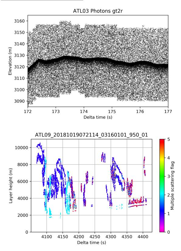
As shown in the ATL03 example above, the photon cloud can at times be denser below the surface than above. The phenomenon is due to multiple scattering and can occur over surfaces with heavy blowing snow, such as the example shown here, or over dense fog. Such conditions result in a widening of the surface return, and more photons apparent below the surface. The effect of multiple scattering is more prominent at night when the solar background signal is absent.
