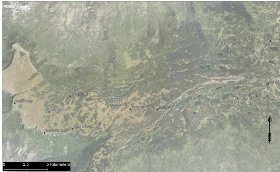
Figure 1. Over the course of the survey, 11 base stations were deployed and occupied for more than 2 hours and used for real-time kinematic (RTK) surveys all over the Mesa. The goal was to have a nearby base station to the active survey so that satellite information was shared across the base and two rover units.
