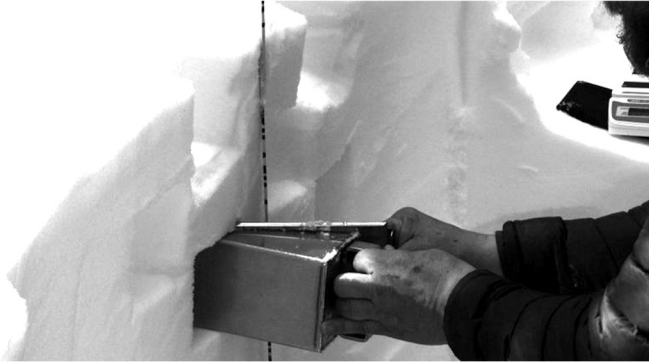
Figure B.7 Simultaneously remove both the sampler and lid to insure no snow loss from the sampler.
