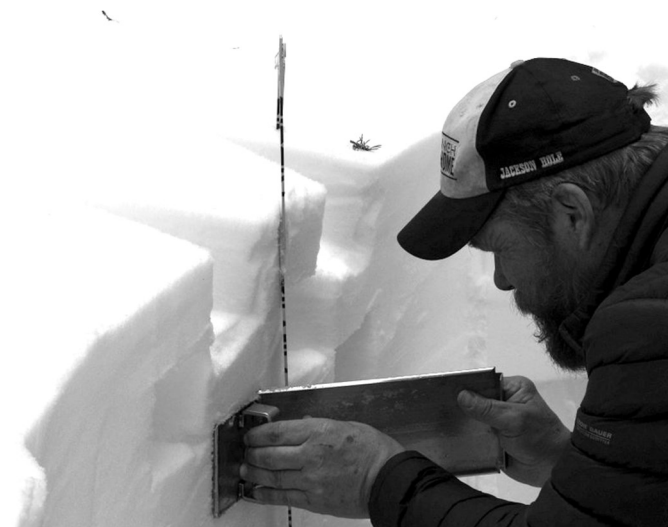
Figure B.6. Hold the sample in the pit wall with one hand while inserting the lid with the other. Angle of insertion is important for the lid to avoid sample error.
