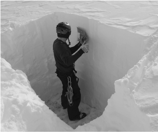
Figure B.2. Carefully shave the pit wall to obtain a smooth surface. This is a critical step for accurate snow density measurements.
