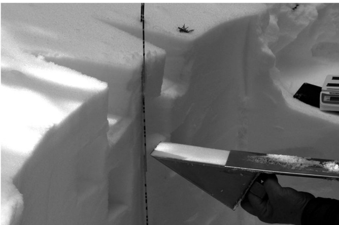
Figure B.8. Slide the lid off the sampler so snow sticking to the inside of the lid is retained in the sample. The lid can then be used to remove snow sticking to the exterior of the sampler in the sides and bottom.
