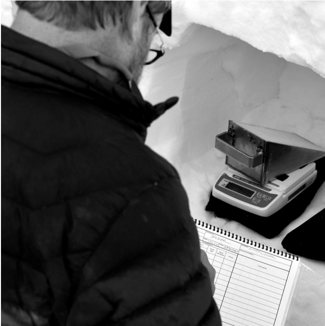
Figure B.9. Weight the clean sample and record the value in the data book.
