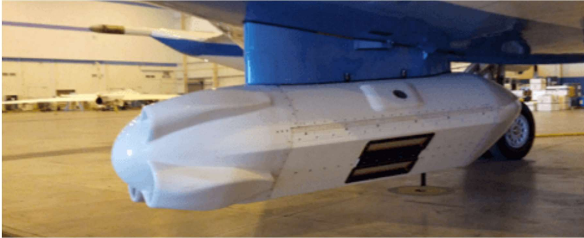
FIGURE 3.1: GLISTIN KA-BAND INSAR INSTRUMENT
