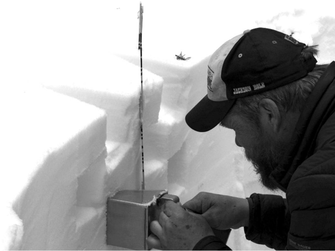
Figure B.5. Carefully line the sampler up so the back plate is parallel to the pit face in all directions when fully inserted.
