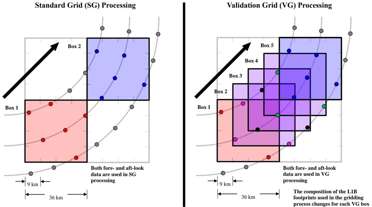
Figure 5.1. Illustration of validation grid processing. The EASE GRID2 boxes are shifted by 3 km increments (although 9 km shifts are shown for clarity) to allow a better geographical match with the *in situ* validation sites.
