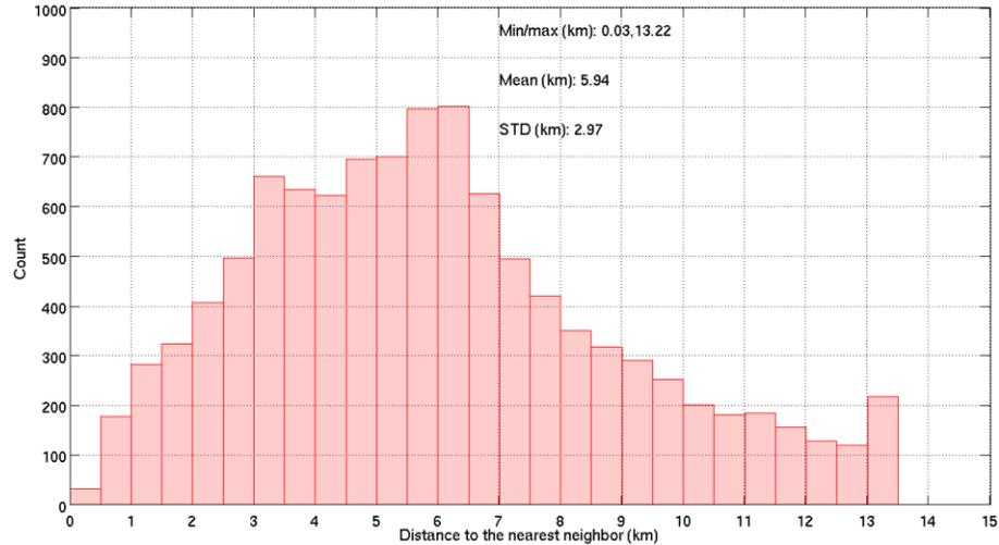
Figure 7.2. Distribution of the shortest distance ( $L_{\min}$ ) between any given sampling location and its nearest neighbor. Based on the actual sampling locations as reported in the ephemeris data of an actual half-orbit L1BTB granule, the mean  $L_{\min}$  was found to be about 6 km with a standard deviation of about 3 km.
