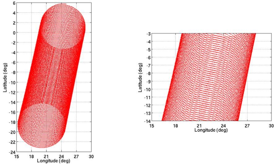
Figure 7.1: Sampling pattern of the SMAP radiometer as reported in the ephemeris data of an actual half-orbit L1BTB granule (left). A closer inspection (right) of the actual sampling locations reveals that over-sampling is achieved in the along-scan direction by virtue of the rotation rate of the SMAP reflector and the integration time of the radiometer.
