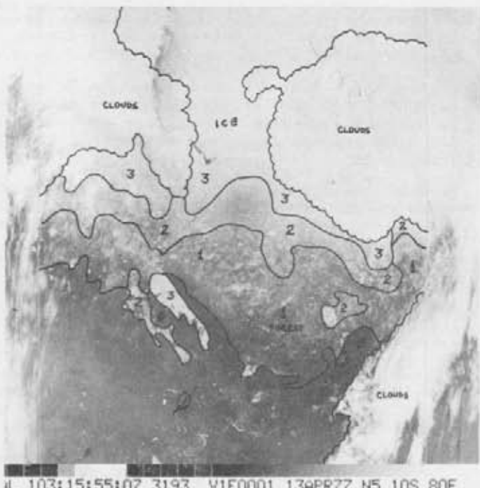
IL 103:15:55:07 3193 VIF0001 13APR77 N5 10S 80E Figure 4. Reflectivity versus ground cover in eastern Canada. Note low reflectivity of densely forested zones with snow on the ground.
