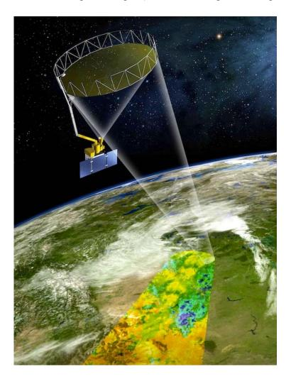
**Figure 1**: The SMAP mission concept consists of an L-band radar and radiometer sharing a single spinning 6-m mesh antenna in a sunsynchronous dawn / dusk orbit.
