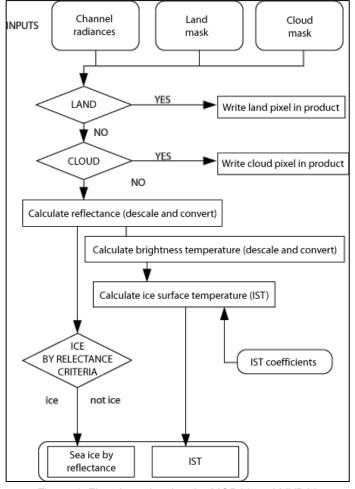
Figure 4. Flowchart showing the MOD29 and MYD29 sea ice algorithm
