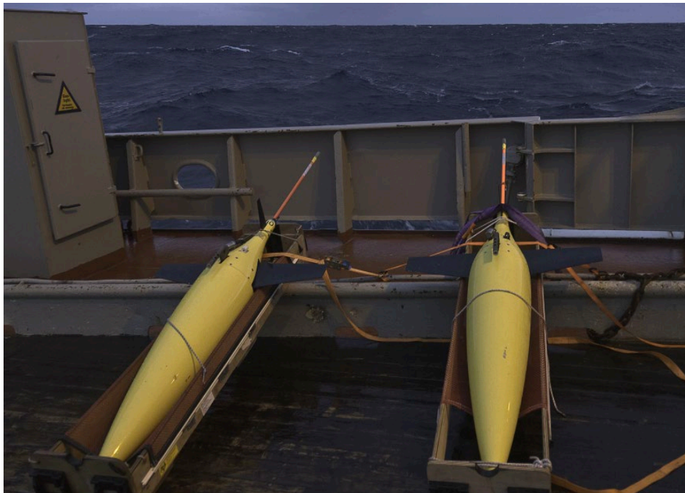
Figure 4. APL-UW ice-capable Seagliders . Gliders navigate survey patterns while diving from the surface/ice–ocean interface to depths up to 1000 m. Figure from Lee et al. (2012).
