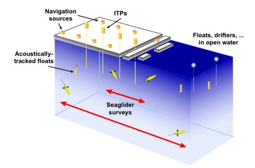
**Figure 9.** The Mobile MIZ Observing Network. Ice-Tethered Profilers, ice-capable Seagliders, and profiling floats, with an acoustic array providing under-ice geolocation and navigation, provide high spatial and/or temporal resolution ocean measurements in the MIZ. The array follows ice drift and retreat though the melt season. Gliders sample from open water, through the MIZ, and into full ice cover, profiling from the ice—ocean interface to 1000 m depth.
