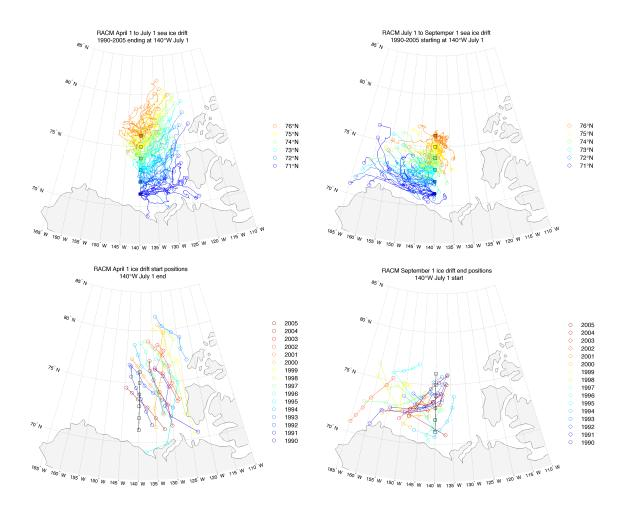
**Figure 6.** Simulated trajectories (1990–2005) derived from analysis of the Naval Postgraduate School's fully coupled Regional Arctic Climate Model (RACM). Back-calculated trajectories (upper left) and starting positions (lower left) from the target 70°–76°N, 140°W line from 1 July to 1 April and forward trajectories (upper right) and end positions (lower right) from the target line on 1 July to an endpoint on 1 September.
