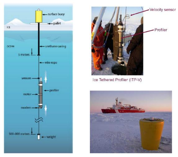
**Figure 8.** Schematic of the WHOI Ice-Tethered Profiler system (left), the profiler with velocity sensor (ITP-V) prior to deployment (upper right), and the surface expression (lower right).
