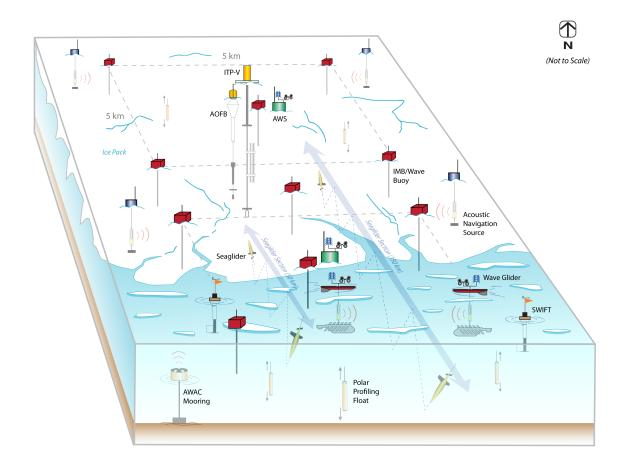
**Figure 5.** Ice-edge and '5-dice' IMB/WB sub-array configuration, depicting oceanographic sampling by floats and gliders beneath the ice and by various ice-based instruments that penetrate through the ice. Gliders conduct sections that extend from full ice cover, through the MIZ, and into open water. Wavegliders and SWIFT drifters sample within the MIZ and the open water to the south.
