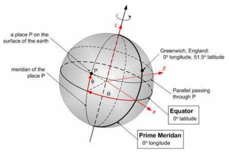
Figure 3: Earth Centered Rotating Coordinate System
