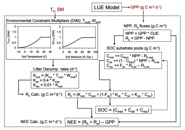
**Figure 4b**. L4\_C terrestrial carbon flux model for estimating NEE. Primary algorithm inputs (in red) include daily GPP from the LUE model (**Fig 4a**), and surface soil moisture (SM) and temperature ( $T_s$ ) from the SMAP L4\_SM product. NEE is the primary (validated) output, while GPP, respiration ( $R_h+R_a$ ) and SOC are secondary (research) outputs.
