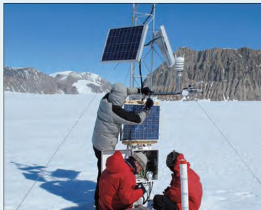
Truffer (in grey), Scambos (left), and Bohlander make repairs on the AMIGOS station on Flask Glacier on the Antarctic Peninsula. (Credit: NSIDC)
