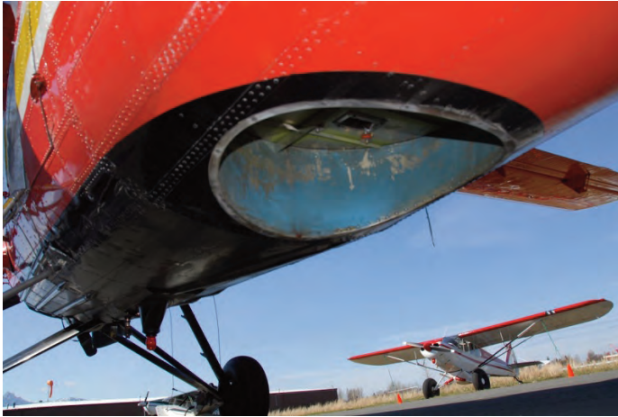
IceBridge utilizes equipment on aircraft to collect data on ice sheets, such as this laser altimeter mounted on a Turbine Single Otter aircraft in Alaska. Credit: NASA Earth Science Project Office
