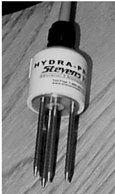
Figure 53. The Hydra probe used at the tower locations.
