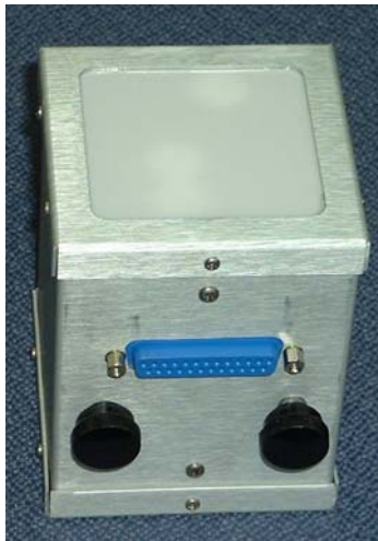
Figure 54. CROPSCAN Multispectral Radiometer (MSR). (Size is 8 X 8 X 10 cm).
