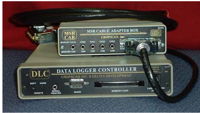
Figure 55 – data logger controller & cable adapter box.
