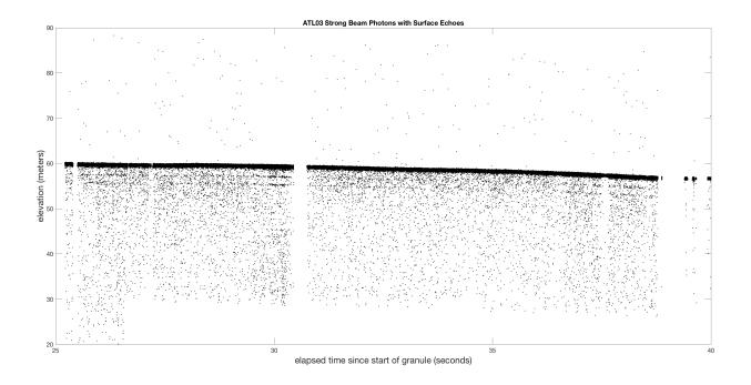
Over relatively flat surfaces, when plotting ATLO3 as along track distance or time, double echoes are sometimes seen at ~2.3m below the primary surface and ~4.2m below the primary surface return. The amount of energy in these additional horizons are typically 1/1000 of the energy in the surface echo. The double echoes appear visually prominent in plots, such as above, because all of the surface return photons are stacked on top of one another, given little changes in photon density.
