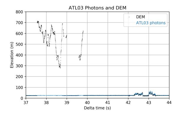
In release 002 and later, the ATL03 product includes the best-available reference digital elevation model (DEM) heights at the reference photon location. The DEM heights reported are prioritized by source: ArcticDEM, Reference Elevation Model of Antarctica (REMA), Global Multiresolution Terrain Elevation Data (GMTED), then DTU13 Mean Sea Surface (MSS). In release 004 and later, GMTED is replaced by the Multi-Error-Removed Improved-Terrain (MERIT) DEM.
