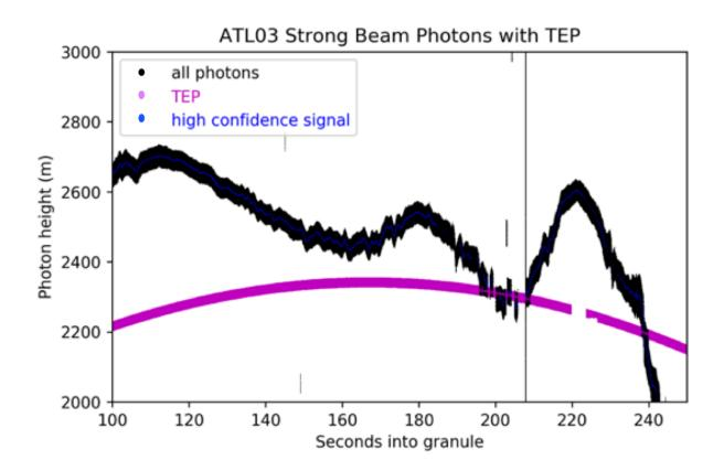
The example above has all telemetered photons in the ATLO3 granule (black), high-confidence signal photons (blue) and an obvious arc passing through the granule just below the apparent surface return.
