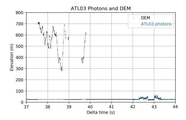
In release 002 and later, the ATL03 product includes the best-available reference digital elevation model (DEM) heights at the reference photon location. The DEM heights reported are prioritized by source: ArcticDEM, Reference Elevation Model of Antarctica (REMA), Global Multiresolution Terrain Elevation Data (GMTED), then DTU13 Mean Sea Surface (MSS).
