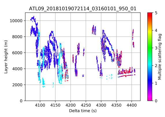
As shown in the ATLO3 example above, the photon cloud can at times be denser below the surface than above. The phenomenon is due to multiple scattering and can occur over surfaces with heavy blowing snow, such as the example shown here, or over dense fog. Such conditions result in a widening of the surface return, and more photons apparent below the surface. The effect of multiple scattering is more prominent at night when the solar background signal is absent.
