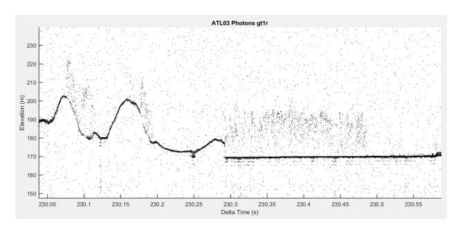
Over flat water, at times the returning laser light will be specular or nearly so. In these cases, the returning laser light will have had minimal pulse spreading and minimal energy loss from light scattering out of the receiver field of view. The returning pulse is therefore narrower and stronger than ATLAS was designed to handle. In these circumstances (e.g. 230.3 to 230.55 seconds), ATLAS detects multiple surface returns, with echoes spaced by either one or two times the ATLAS dead time.
