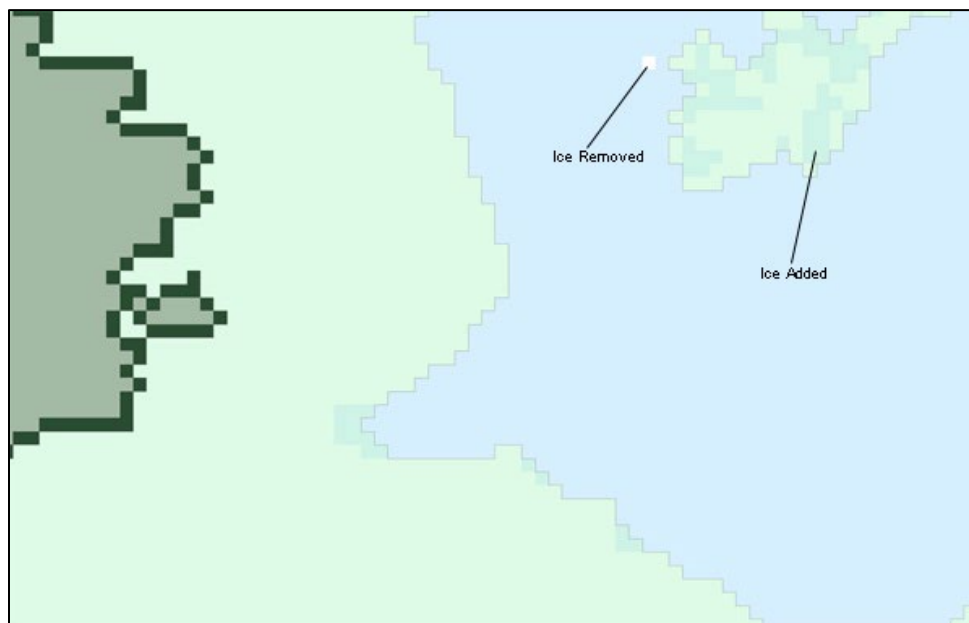
Figure 8. Illustration of Closing Operation: The medium green on the left side is land; the dark green surrounding it is coastline. The area of the lightest green is the sea ice area prior to the closing operation. The light green within the lightest green is sea ice added during the closing operation. The single stand-alone white cell was marked as sea ice in the input IMS product, but is eliminated when sea ice polygons smaller than 16 cells, or roughly 256 sq km, are discarded. The grey line around the light and lightest green is the smoothed ice edge.
