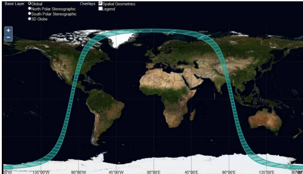
Figure 1. Spatial Coverage Map displaying one orbit of the Aquarius Radiometer. The map was created using Reverb | ECHO .
